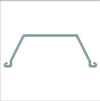
$I_y = 2.12E-04 \text{ m}^4/\text{m}$ ;  $A = 1.49E-02 \text{ m}^2/\text{m}$ ;  $E = 210000.00 \text{ MPa}$ ;  $G = 81000.00 \text{ MPa}$
